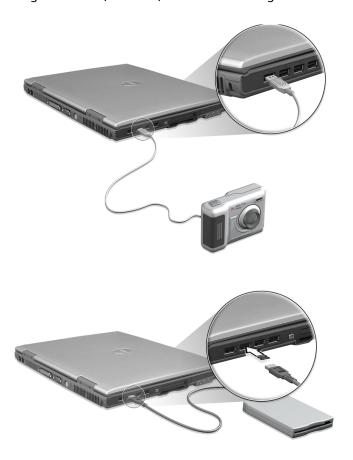
USB is plug and play, which means that you can connect and start using a USB device without having to restart your computer. You can also disconnect the device at any time.
